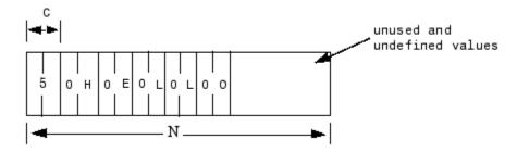
These serial blocks interpret each entry in the vector as a single character. The low-level Send block writes the low-order byte of each entry to the UART. The 16-bit and 32-bit data types allow the embedding of 8-bit data values, including  $\theta$ . The 8-bit data type is most useful with the ASCII Encode and Decode blocks. The 16-bit and 32-bit data types are most useful for binary data streams.
